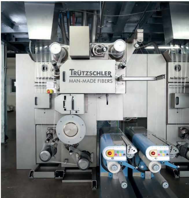
The 4-filament BCF extrusion system MO40
